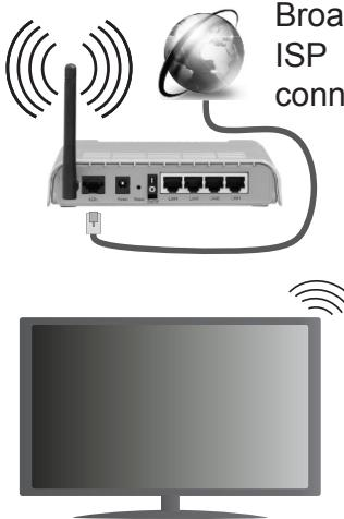
A Wireless-N router (IEEE 802.11a/b/g/n) with simultaneous 2.4 and 5 GHz bands is designed to increase bandwidth. These are optimized for smoother and faster HD video streaming, file transfers and wireless gaming.
