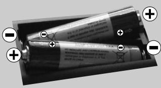
Remove the screw that secure the battery compartment cover on the back side of the remote control first. Remove the cover gently. Insert two **AAA** batteries. Make sure the (+) and (-) signs match (observe correct polarity). Do not mix old and new batteries. Replace only with same or equivalent type. Place the cover back on. Then screw the cover back on again.
